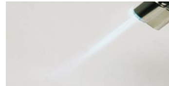
Additionally for marble and limestone: Expose the surface to flame treatment (to produce a SiOx layer)
